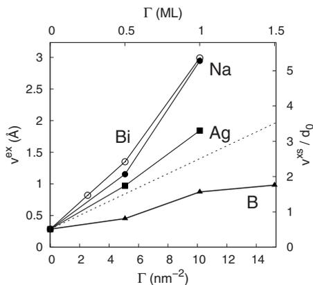
FIG. 5. The grain boundary excess volume per unit area,  $v^{xs}$ , as a function of impurity excess  $\Gamma$ . Data for Bi, Na, and Ag are from Ref. 8. The right hand scale gives  $v^{xs}$  in units of  $\{310\}$  interlayer spacing in bulk copper,  $d_0=0.5576$  Å. The dotted line corresponds to a hypothetical ideal impurity identical with Cu atoms.
