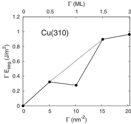
FIG. 3. Convex hull plot for B impurity at the Cu(310) surface. Circles correspond to the lowest energy surfaces for each coverage found in our study. According to these, the energy of the system is lowered if ordered unreconstructed 1 ML surface decomposes into 0.5 ML and 1.5 ML surfaces (dashed line).
