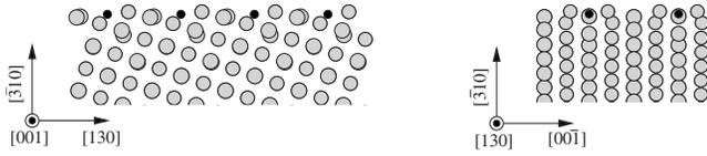
FIG. 7. Two side views of the relaxed Cu(310) surface with 0.5 ML of boron. Boron atoms were initially placed instead of the top layer of Cu atoms from which every other atom along the [001] direction was removed. During the relaxation, boron atoms descend below the next Cu layer causing a noticeable distortion of the latter.
