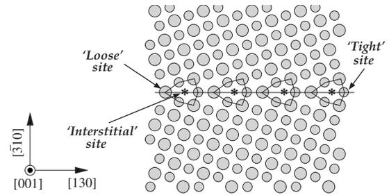
FIG. 2. Equilibrium structure of the  $\Sigma 5\{310\}[001]$  symmetric tilt grain boundary in pure copper. Larger and smaller circles represent alternating (001) Cu planes. The grain boundary plane contains two inequivalent Cu atoms which we refer to as the loose and tight sites. The interstitial site suitable for segregation of small impurity atoms is shown with an asterisk.
