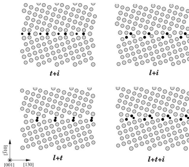
FIG. 6. Relaxed  $\Sigma 5$  copper grain boundary with 1 and 1.5 ML of boron. For 1.5 ML, boron occupies loose, tight, and interstitial sites at the grain boundary plane. For 1 ML, any two of them are occupied (three combinations). Works of separation and grain boundary excess volumes corresponding to these boundaries are listed in Table III. Larger and smaller circles correspond to host and impurity atoms lying in neighboring (001) planes.
