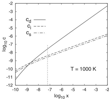
FIG. 8. Equilibrium concentration of  $B_d$ ,  $B_i$ , and  $B_s$  in  $\text{Cu}_{1-x}\text{B}_x$  at  $T=1000$  K given by Eqs. (A12) and (A13) as a function of boron content  $x$ . The vertical dotted line corresponds to the solubility limit  $x^m$  estimated according to Eq. (A16).
