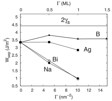
FIG. 4. The work of separation of the  $\Sigma 5(310)[001]$  Cu grain boundary,  $W_{\text{sep}}$ , as a function of impurity excess  $\Gamma$ . Data for Bi, Na, and Ag are from Ref. 8. The horizontal line corresponds to twice the surface energy of Cu(310) (Ref. 8),  $\gamma_s = 2.21 \text{ J/m}^2$ , which provides a natural upper bound for  $W_{\text{sep}}$ .
