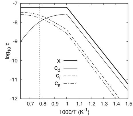
FIG. 9. Equilibrium concentration of  $B_d$ ,  $B_i$ , and  $B_s$  and the total amount of boron,  $x=c_i+c_s+2c_d$ , as a function of  $T^{-1}$  (the Arrhenius plot). The alloy composition is taken as the terminal solution at  $T=1000$  K (vertical dotted line in Fig. 8). The kink on the curves corresponds to the precipitation of the second phase (assumed to be pure  $\alpha$ -B). The vertical dotted line indicates the eutectic temperature  $T_e=1013$  °C.
